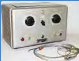
Power unit for one of the first heart pacemakers
